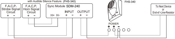
Horn or Strobe Wiring Diagram for Audible Strobe Class "B" Circuit without Audible Silence Feature.
