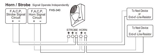
Horn / Strobe Wiring Diagram for Audible Strobe Class "B" Circuit with Audible Silence Feature. (FHS-340)
